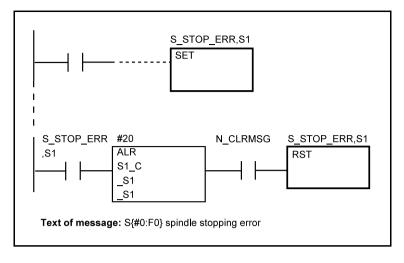
Write the number of spindle also in the text of message: the value of optional variable: S1. The message is fully encoded by the number of channel and spindle. The number of spindle has also taken to text of message to ensure transparency.
