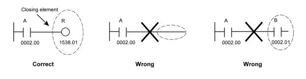
In case of a closing element, you can always define **comment** by filling Remark parameter. The comment is written in the row of closing element, from the column following the closing element.
