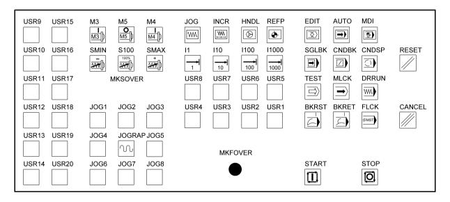
The following symbols of the machine control panel buttons and lamps are all symbols with *bit* reference.
