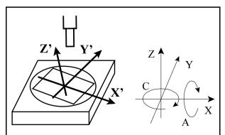
Rot. Ax.=A and N3208 No. of the Second Rot. Ax.=C. In such a case, when X or Y jog button is pushed or Z axis is selected for handwheel moving, the motion will be executed in the plane of the table, taking positions of the A and C axes into account. When Z jog button is pushed or X or Y axis is selected for handwheel moving, the motion will be executed in the direction perpendicular to the plane of the table, taking positions of the A and C axes into account.
