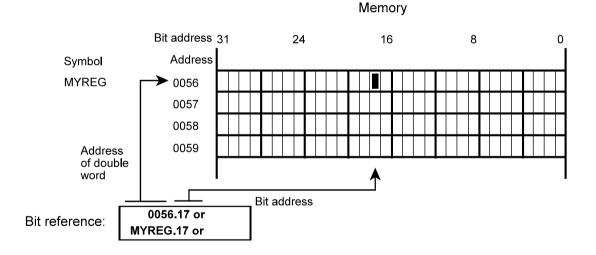
If you have a declared symbol for a bit address, then you can refer directly to bit by **symbol**. For example, if you have declared DRV\_RDY symbol to bit address 0117.09, then you can reach the bit 0117.09 directly by
