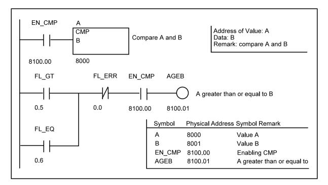
The following figure shows how to evaluate the condition  $A \ge B$  using CMP instruction.
