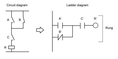
contacts. They can be controlled by inputs/outputs, or they can be the open or closed contacts belonging to internal auxiliary relays, holding relays, timing relays. On the right end of logic line there are "coils" of outputs, timers, counters or instructions.
