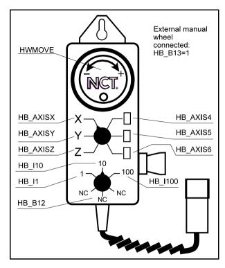
Bit variables of the external handwheel are the following:
