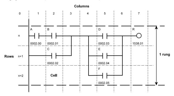
Most of the **instructions**, except some of them, **must not be written directly to the first column**, only after a contact. So, for example, relay coil or SET instruction could not be connected directly to the left side vertical wire.
