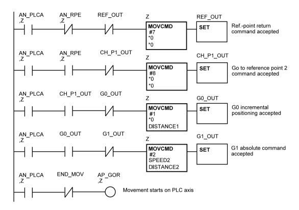
The interpolator immediately takes off the command reference point return from the buffer, therefore flag AN\_BEPTY (buffer is empty) is not changed, so it indicates that the buffer is empty.
