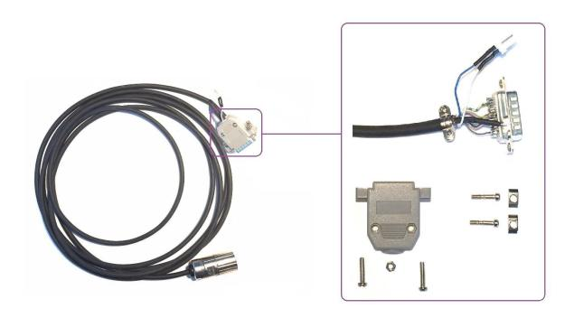
Before assembling the D-SUB connector, place a shrinkable tube of  $\varnothing 30$  mm nominal diameter on the cable for later clamping the assembled cable and the assembled battery.
