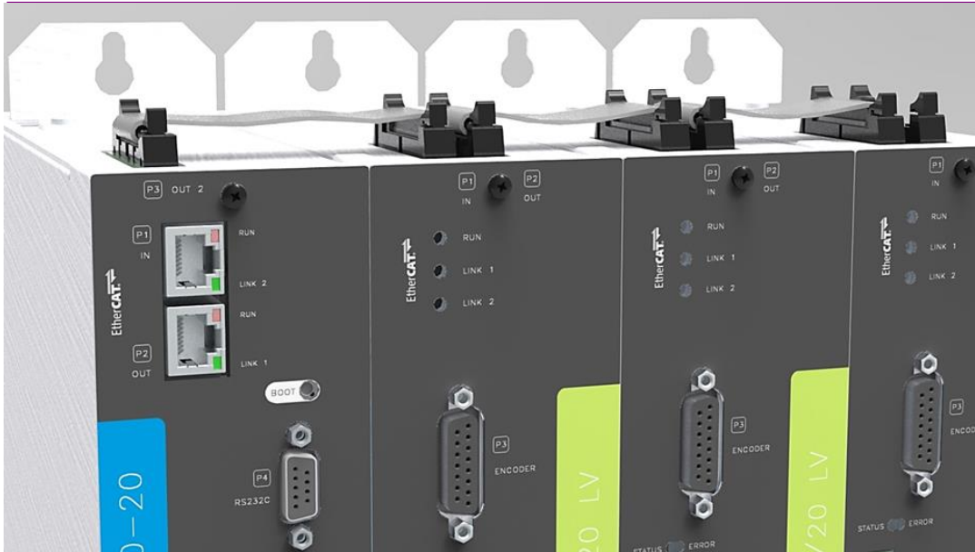
Figure 2 LVDS flat cable chaining
