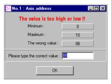
not in the latent range of the parameter. Then the pop-up window informs us about the parameter which can be seen in he header, and its minimum/maximum value and the incorrect value written by us. The window cannot be closed unless we write in the correct value. After giving the correct value and pressing OK we can continue
