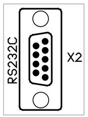
The programming of DPB.. supply unit is possible by means of IBM compatible personal computers (PC). In this case the DPB.. supply unit must be connected to the computer. Shielded cable must be used for the connection, shielding must be soldered to the connector casing on both sides.
