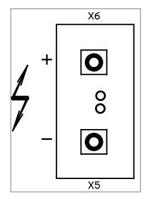
DC voltage connection points of NCT servo drives and supply units are equally far from the mounting plate, thereby copper bus can be used for connecting modules. In case it is not possible, copper cable supported with cable-eye can be applied. The cross-section of the copper cable must correspond with the cross-section of line cables of the supply unit.
