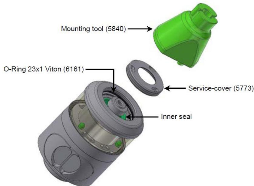
**Figure 13 Maintenance and cleaning of infrared touch probe IRP40.02**
