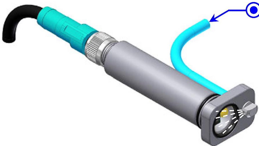
Figure 19 Cleaning the glass pane
