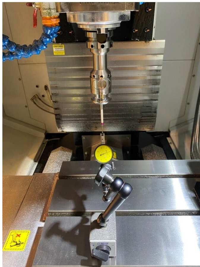
Figure 1 Relationship between the workpiece gauge and the dial gauge
