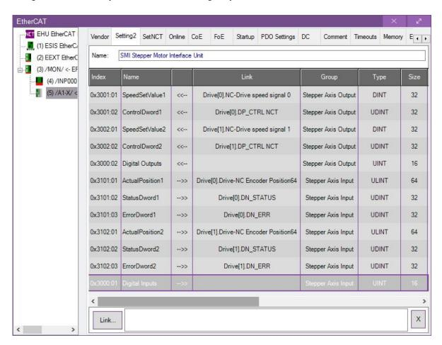
The picture above shows that the axis 1 of the module being STEPPER mode has been assigned to the drive 0 and its axis 2 to the drive 1; the digital input and output variables have not been assigned to PLC symbols.
