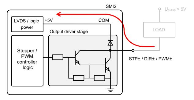
All the open collector outputs (STP±/DIR±/PWM±) have the same output driver stage which is shown on picture above (only one output is shown). Do not apply higher pull up voltage than 5V because an undesired balancing current can be flown form the pullup power supply into the SMI2 via the free running diode of the output drive stage.
