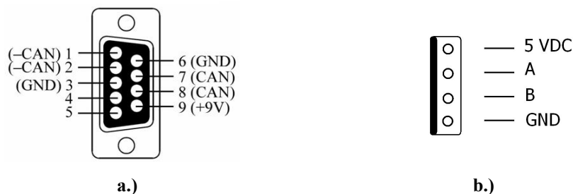
Fig. 3 Connectors of the machine keyboard handwheel: a.) CAN bus handwheel connector, b.) incremental handwheel connector
