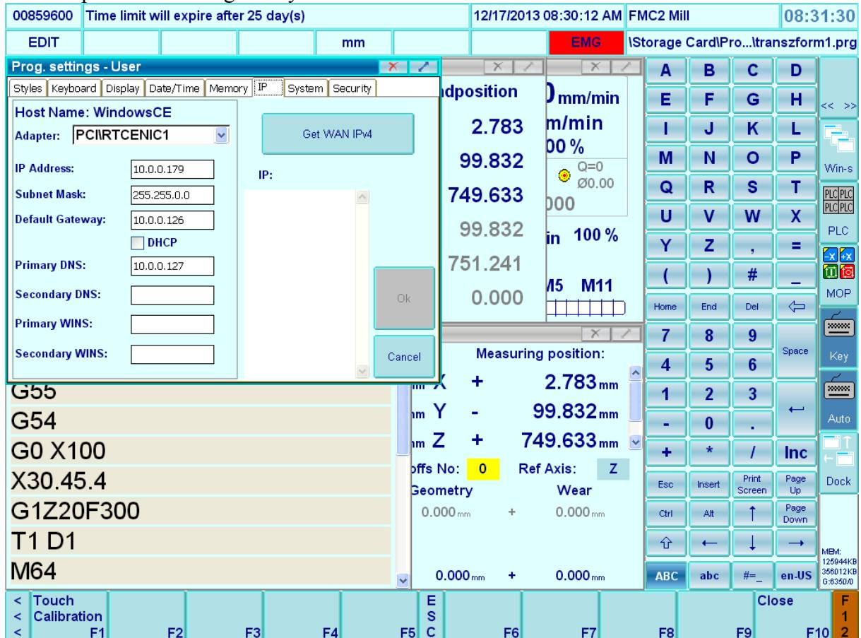
After you change this setting, you need to restart the controller. (Switch off and on the machine, not enough to restart the software only)
