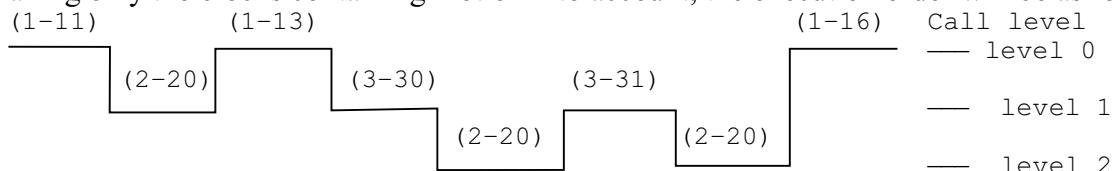
The first of the numbers in parentheses means the number of the program being under execution, and the second one means the number of the block being under execution.
