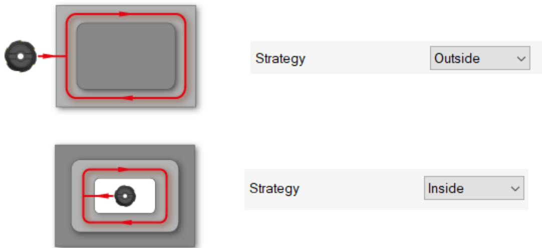
7-11. Figure Strategy: milling from outside or from inside
