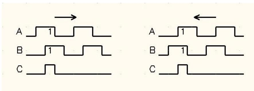
The correct setting should be checked in both directions of rotation!
